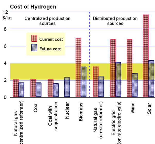
Figure 4: Hydrogen production cost
