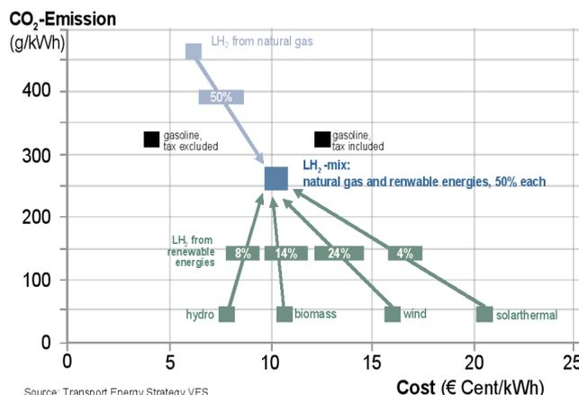
Figure 5: LH<sub>2</sub> costs and CO<sub>2</sub> emissions – dissimilar energy pathways compared
